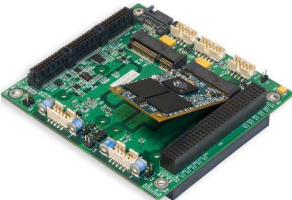
Fig. 4-1: Installation of additional Mini PCI-E cards into a relevant connector
