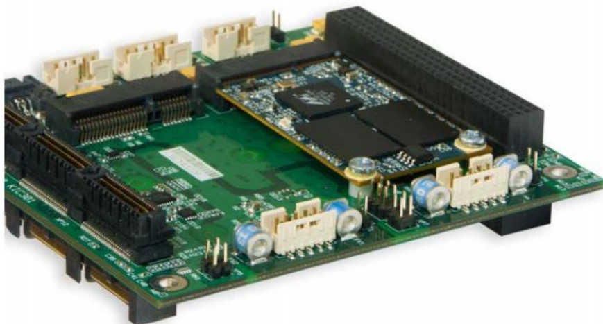
Fig. 4-3: KIC301 with the installed Mini PCI-E card
